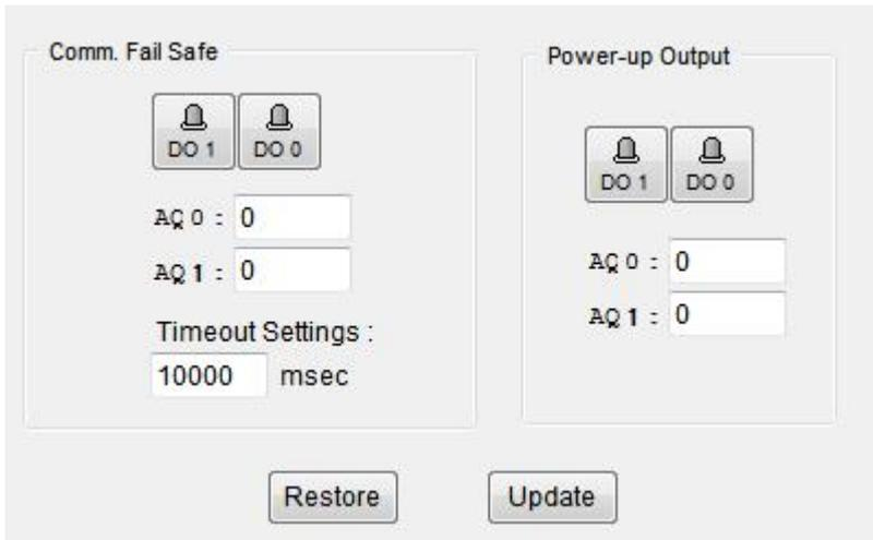
9. When turn on the Remote IO Module's power, can set the power on output indicator via **Power On Digital Output**. When finish it, press Update to save. Or can click Restore to restore device's current data.
