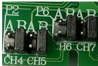
Thermistor: Pin B short
